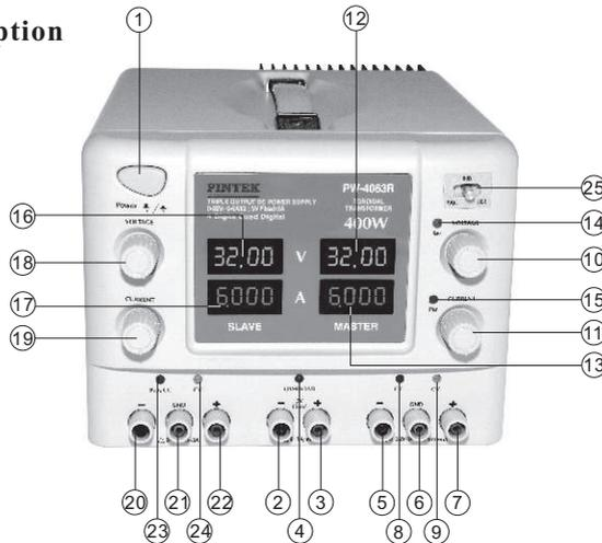
1. **Power switch:** Push the switch button to turn "ON" the power and the LED(12,13,16,17) will light up; to push the button again, to turn it "OFF" .
