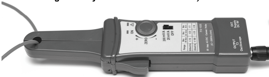
Figure 2: Connecting the PA-659 current probe.
