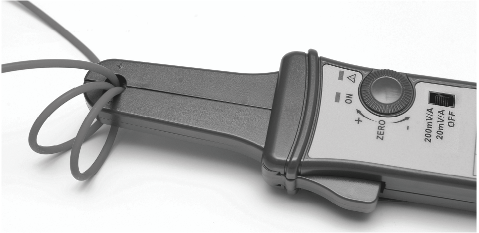
Figure 4: Increasing the sensitivity
