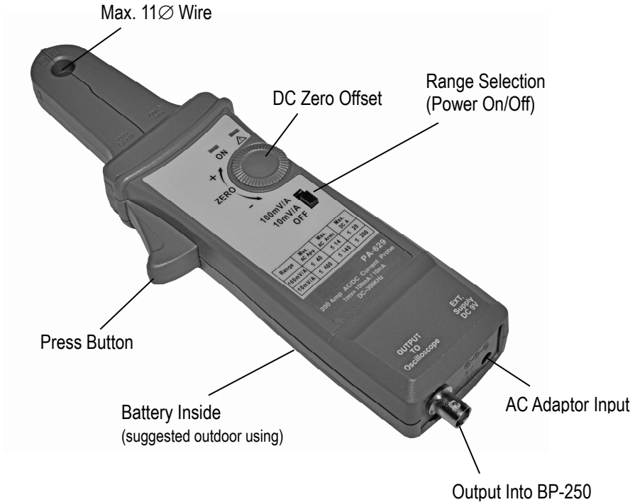
Figure 1: shows the controls and indicators on the PA-629 current probe.
